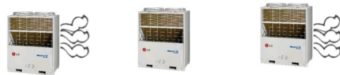
Full defrost Normal operation Full defrost
