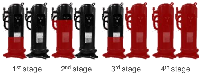
Compressor sequence control
