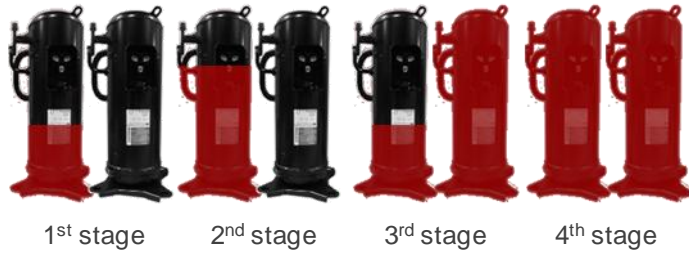
Compressor sequence control
