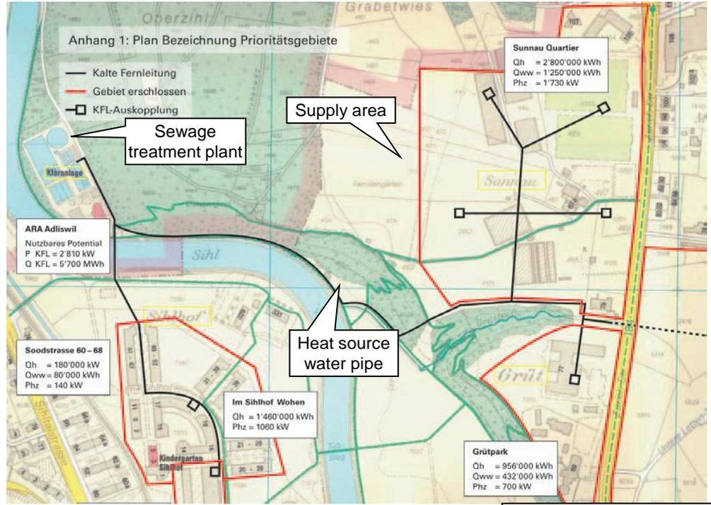
This network system consists of low temperature heat source water line to conduct heat exchange with the effluent from ARA (sewage treatment plant).
