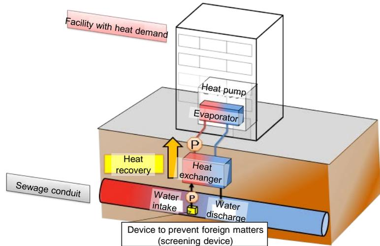
Outside-of-conduit type heat exchange method for heat from untreated water
