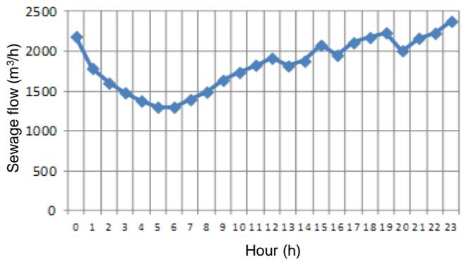
Example of sewage conduit flow measurement in **residential areas** (total floor area of houses occupies 72%)
