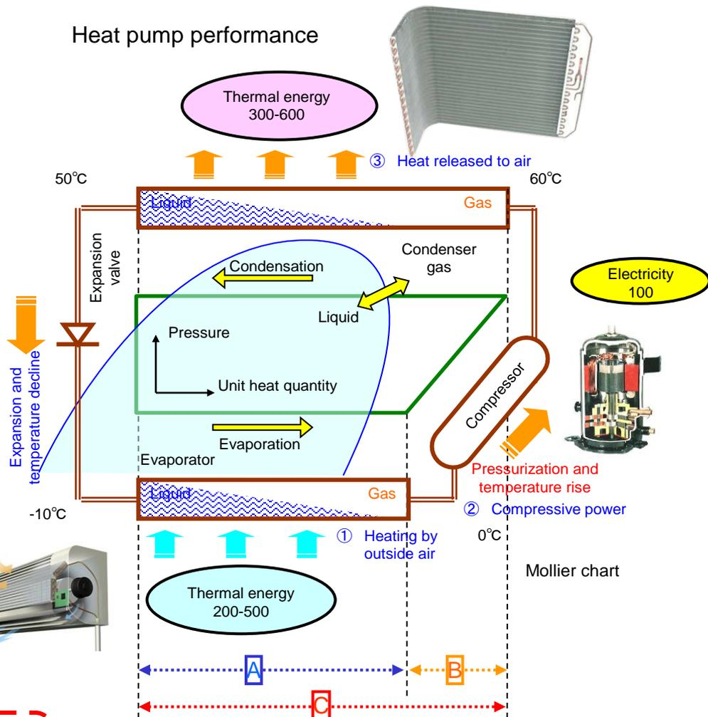
In case of heating: Temperature of each part shows an example and varies depending on operating conditions (volume of refrigerant circulated, air flow).
