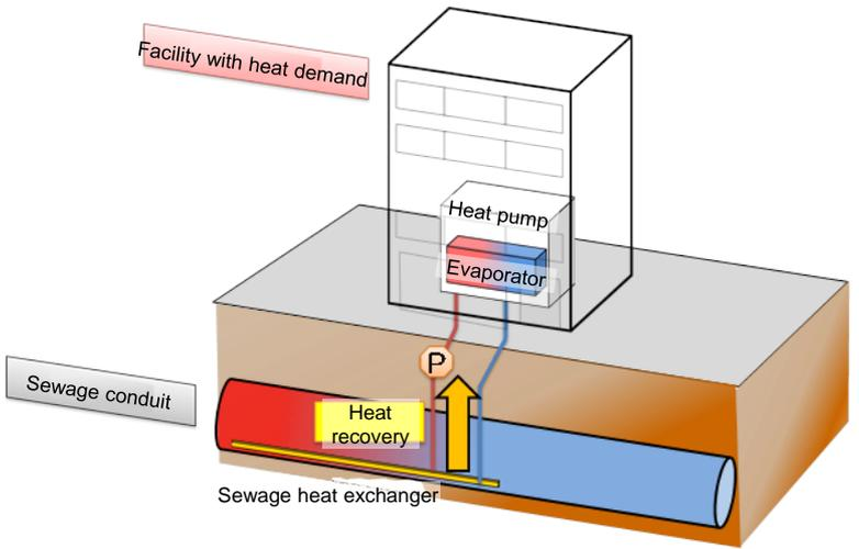
Inside-of-conduit type heat exchange method for heat from untreated water
