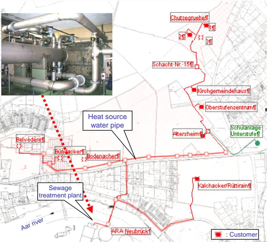
This line consists of low temperature heat source water line to conduct heat exchange with the effluent from ARA (sewage treatment plant). Nearby houses and offices have their own heat pumps.
