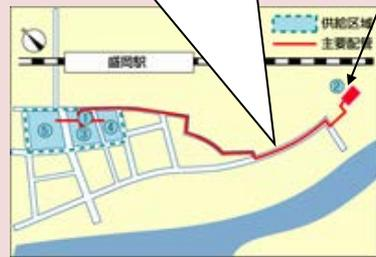
The water treatment plant and heat source plant are connected by the heat source water conduit with a length of about 1 km.
