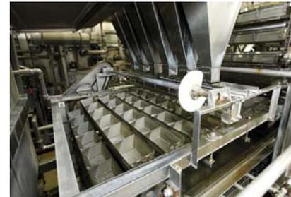
↑ Cooling tank used after the process of boiling noodles
