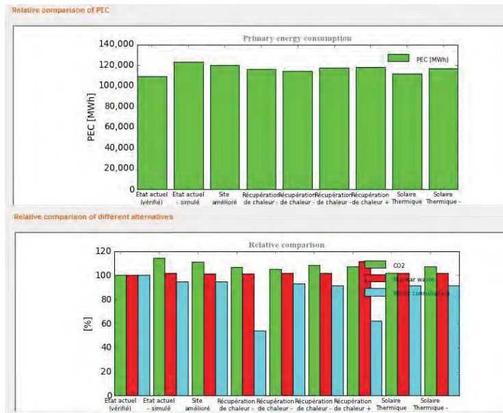
Figure 3-19: Comparison of various scenarios depending on primary energy consumption (top graph) and environmental impacts - CO 2 , nuclear waste, water consumption (bottom graph)
