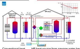
HP heat source from sewage water heat (during heating) Bypass operation in summer
