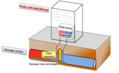
Inside-of-conduit type heat exchange method for heat from untreated water
