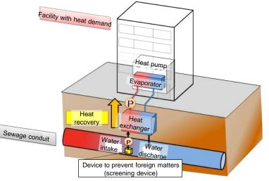
Outside-of-conduit type heat exchange method for heat from untreated water
