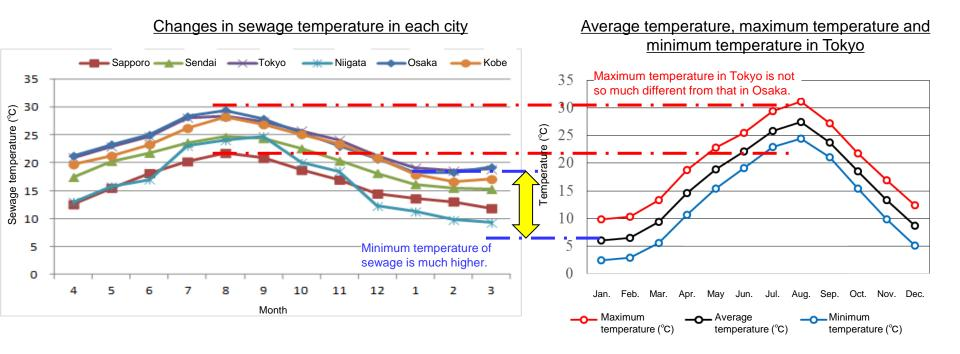
Sewage temperature in Sapporo is advantageous to obtain heat for heating and hot water supply in winter as well as heat for cooling in summer.
