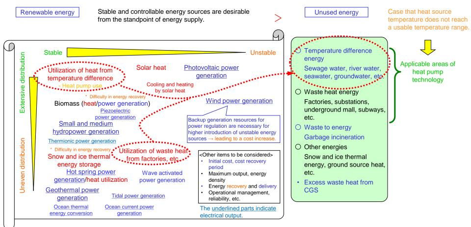
Outputs of photovoltaic power generation (national average utilization rate: 12%) and wind power generation (national average utilization rate: 20%) change significantly.
