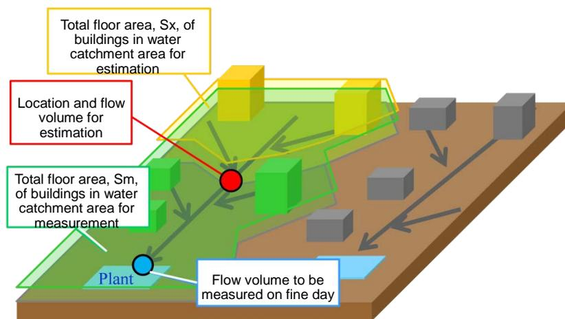
Figure 21: Sewage flow volume estimation method
