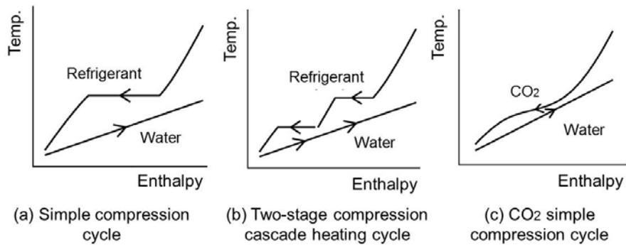
Fig.2 Comparison of heating cycle (Temperature - Enthalpy Diagram)
