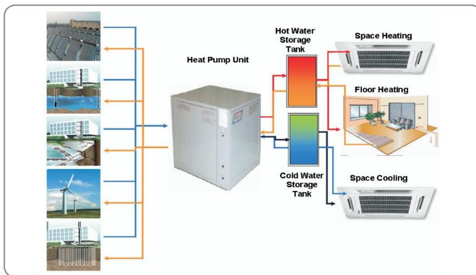
**Figure 4. High efficient heat pump water heater with hybrid source**
