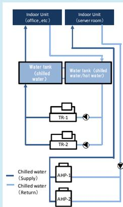
In this facility, two turbo refrigerator and two air source heat pump chillers are operated.
