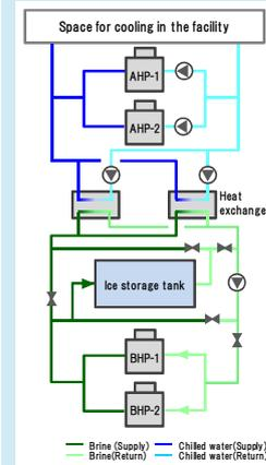
In this facility, two air source brine heat pumps (BHP-1,2) are operated at night to store cold heat in the tank of internal ice melting system. Cold heat in the tank and two air source heat pump chillers (AHP-1,2) provide cold heat for space cooling in day time.
