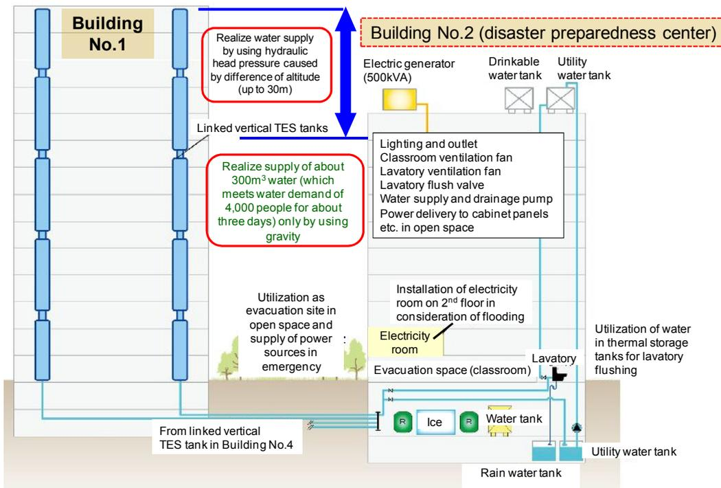
Figure 8: TES tank utilization scheme in case of emergency (Tokyo Senju Campus of TDU)
