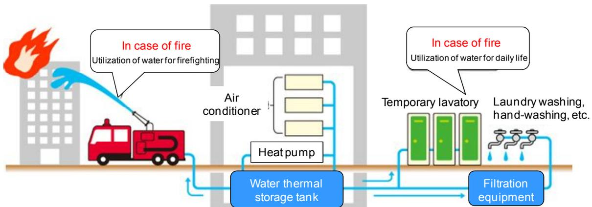
Figure 6: Image of thermal storage tank utilization in case of emergency
