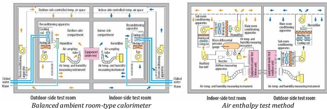
**Figure 1: Examples of air conditioner performance testing facilities**
