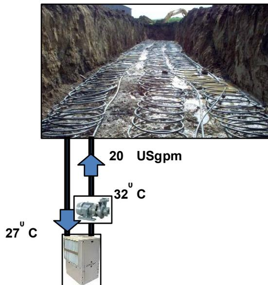
Figure 2: Geo-exchange System
