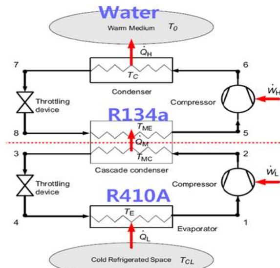
Figure 7. Cascade cycle refrigeration
