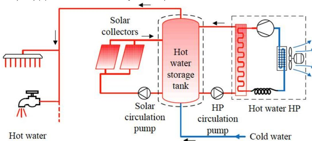
Figure 1. Schematic diagram of the combined systems
