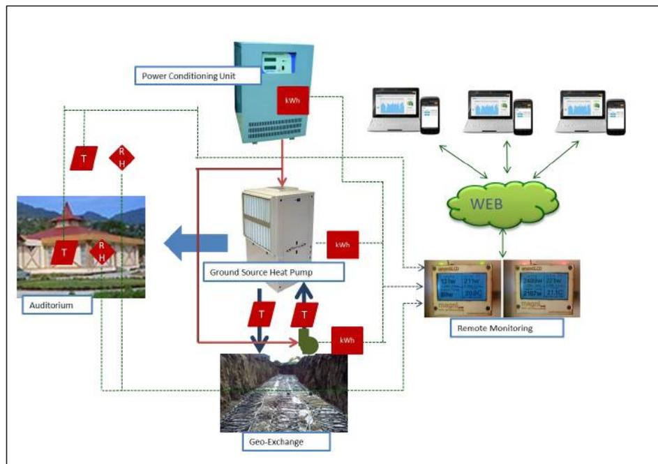
**Figure 4: Remote Monitoring System**
