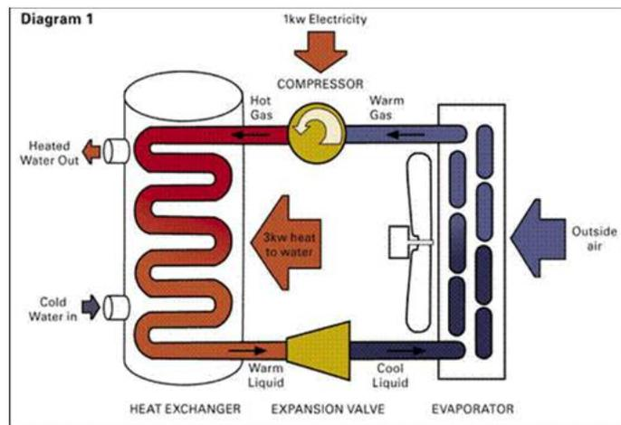
Figure 2. Basic cycle of refrigeration cycle for heat pump water heater
