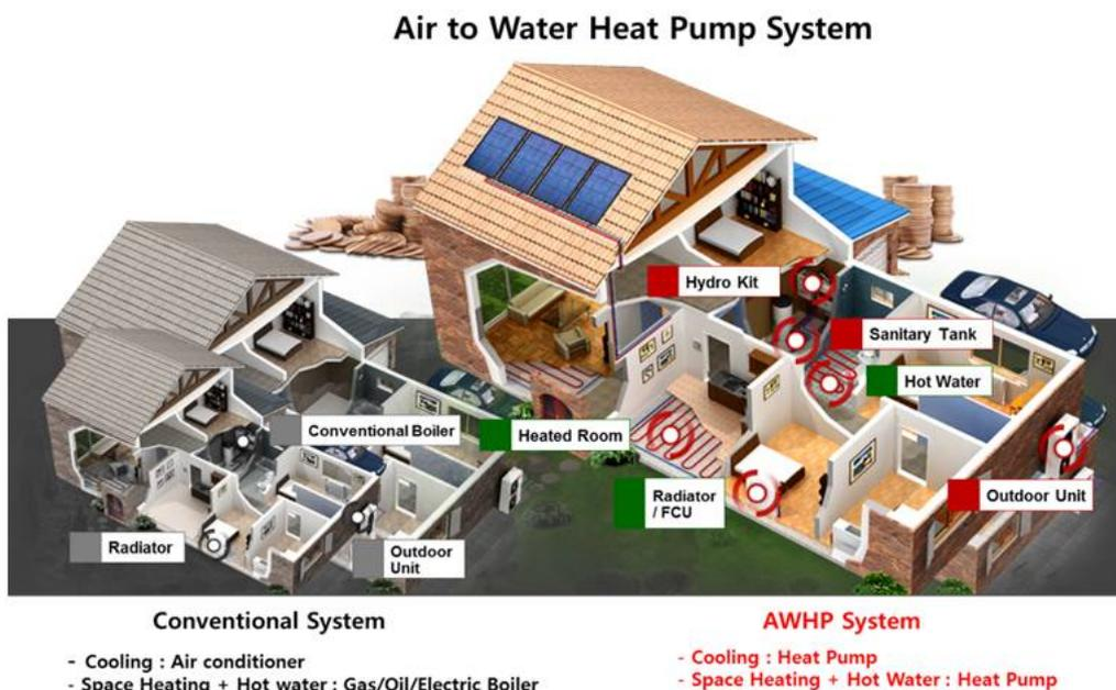
**Figure 1. Installation of domestic air source heat pump water heater**
