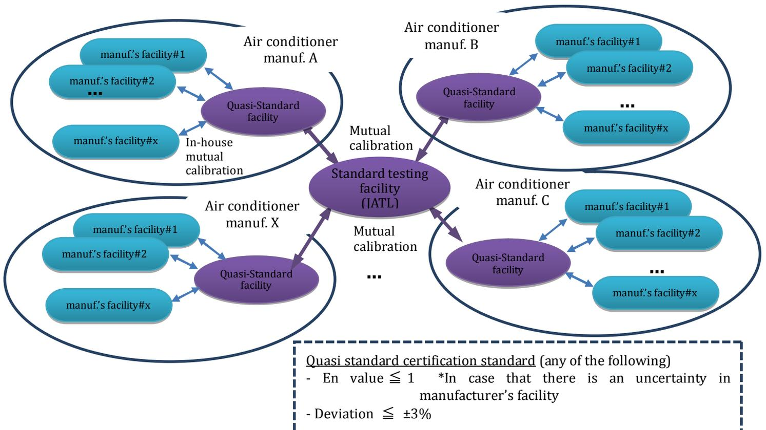
Figure 4: Scheme of quasi standard certification in verification system
