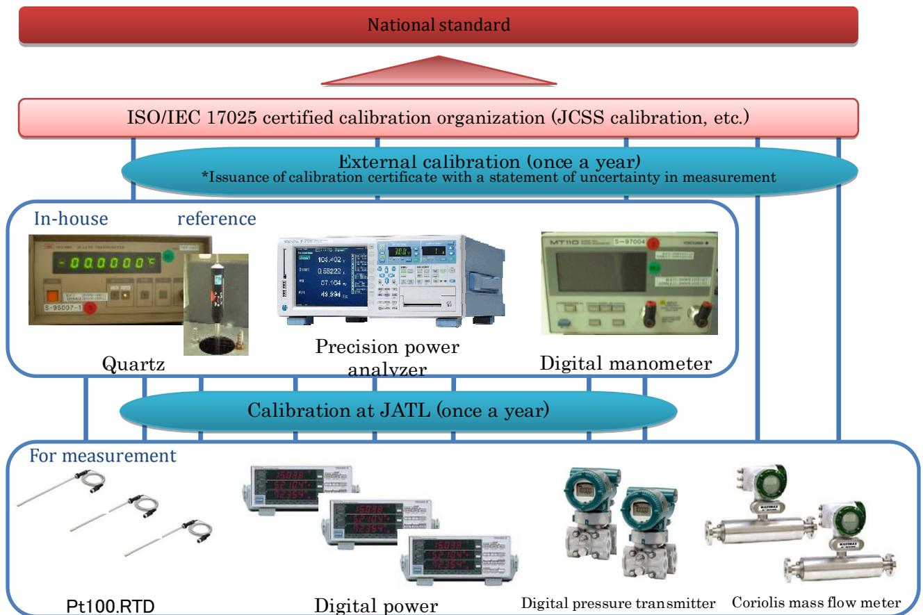
Figure 2: Traceability diagram of measuring instruments (excerpt) at JATL
