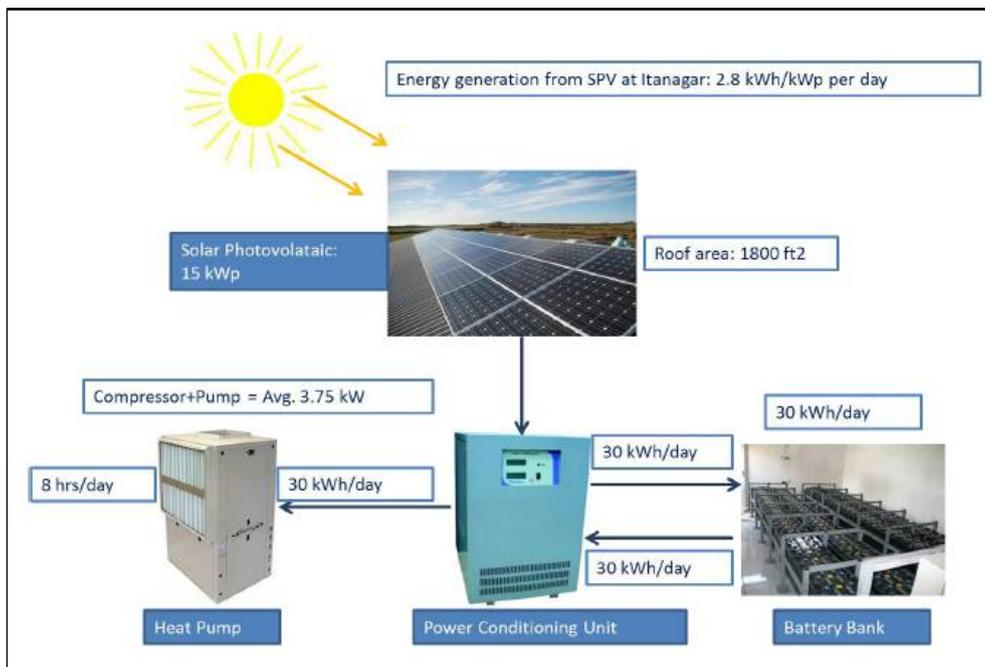
**Figure 3: Solar Photovoltaic System**
