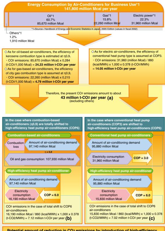
Potential amount of reduction in CO<sub>2</sub> emissions by introduction of high-efficiency heat pump air-conditioners  $\mathbf{a} - (\mathbf{b} + \mathbf{c}) =$  about 29 million t-CO<sub>2</sub> per year
