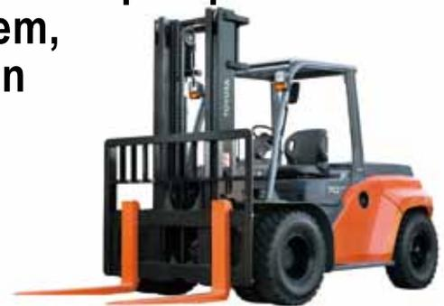
Engine powered forklift
