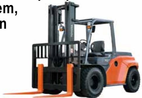
Engine powered forklift
