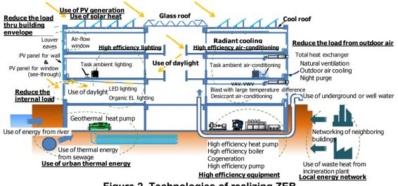
Figure 2. Technologies of realizing ZEB
