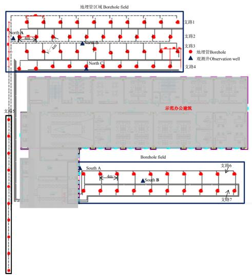
Figure 3. Borehole System distribution
