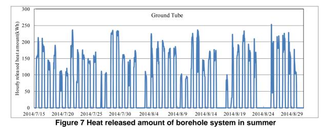
Figure 7 shows hourly heat release amount of borehole ground-tube, a maximum hourly release heat amount of about 220kWh with an average is about 120 kWh was found in the figure, accumulated released heat amount is about 54000kWh. COP is assumed as 4.0 on average, cooling load of the building is about 4320kWh.
