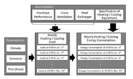
Figure 5 Method of calculating space heating / cooling energy consumption
