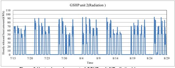
Figure 9 Heat released amount of GSHP unit 2(Radiation) in summer
