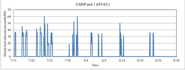
Figure 8 Heat released amount of GSHP1(HVAC) in summer
