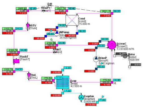
Figure 2. Results from the low stage cycle simulation
