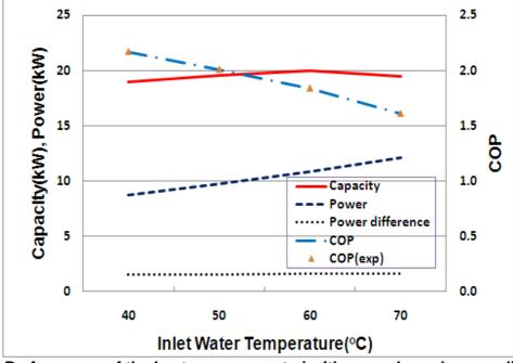
Figure 4. Performance of the heat pump operated with cascade cycle according to hot water inlet temperatures
