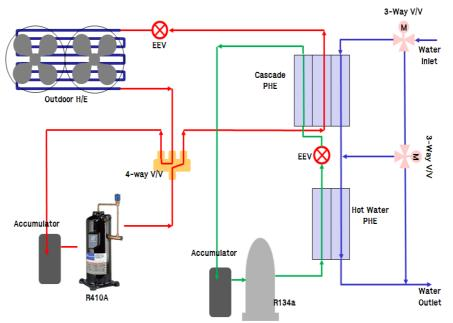
Figure 1. Schematic diagram of the air to water heat pump
