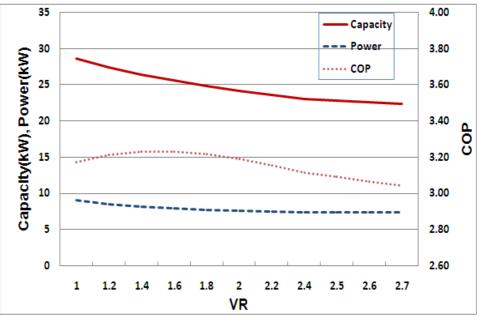
Figure 3. Changes in heat pump performance according to VRs
