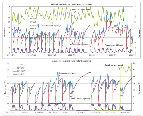
Figure 4 Ground water inlet and outlet temperature variation from July 15th to 30th August
