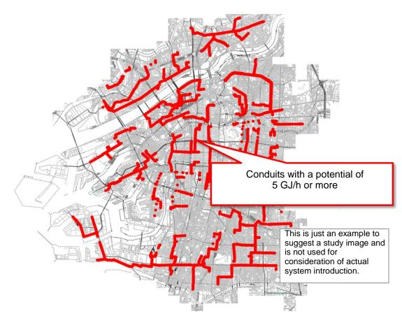
Figure 22: Example of estimation of a potential for sewage heat utilization in trunk sewage conduits of cities
