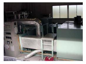
Heating/cooling capacity 5kW, installed in 1999 Fig.6 Test chamber for prototype of CO2 heat pump water heater
