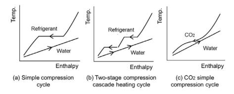
Fig.2 Comparison of heating cycle (Temperature - Enthalpy Diagram)
