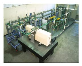
Heating capacity 4kW, installed in 1996 Fig. 5 Basic experiment loop for CO2 heat pump
