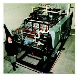
Heating capacity 150kW, installed in 1991 Fig.4 Prototype of two-stage compression system for business use
