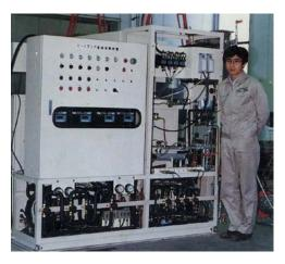
Heating capacity 4kW, installed in 1987 Fig.3 Experimental apparatus of two-stage compression system
