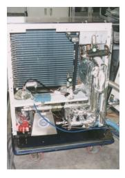
Heating capacity 4kW, installed in 1999 Fig.7 Prototype of CO2 heat pump water heater for residential use
